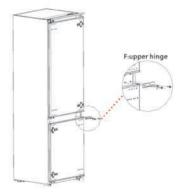
7) Remove the freezer door, the bottom hinge and the hole caps.
