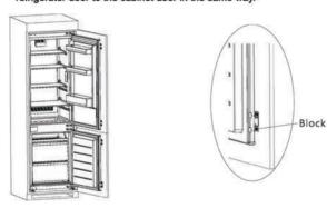
Take out the sealing strip from accessory bag, and press it in the gap between the cabinet and the
