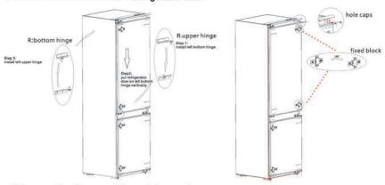
6) Remove the the upper hinge of freezer door.
