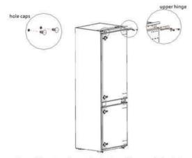
3) Remove the refrigerator door, the bottom hinge and the hole cover.
