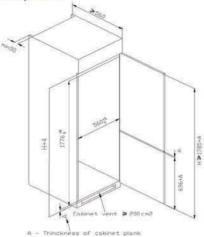
Push the refrigerator into the cabinet and adjust it to make sure the edge fold of top baffle completely
