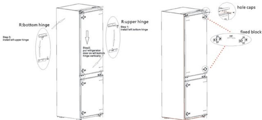
6) Remove the the upper hinge of freezer door.
