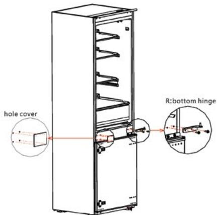
4) Exchange the R:bottom hinge and R:upper hinge , then install them according to below steps, and install the top hole caps.
