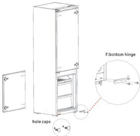
8) Exchange the F:bottom hinge and F:upper hinge , then install them according to below steps, and install the top hole cover and lower hole caps.
